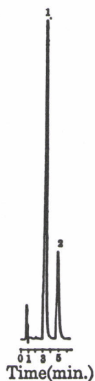
Fig.5. Chromatogram of Oxprenolol HC1 Tablet. (1) Metoprolol Tartrate, (2) Oxprenolol HC1. Conditions : The same as in Fig.1.
