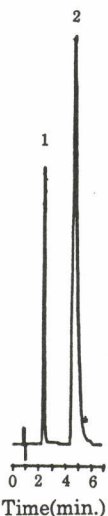
Fig.3. Chromatogram of Pindolol Tablet. (1) Pindolol, (2) Oxprenolol HCl. Conditions : The same as in Fig.1.
